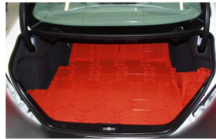
Figure 1: Physical measurement according to DIN 70020
