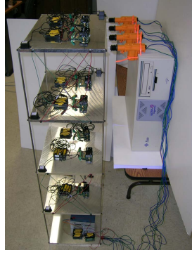
Fig. 5. The 48 inch scaled model of a 4-story building
