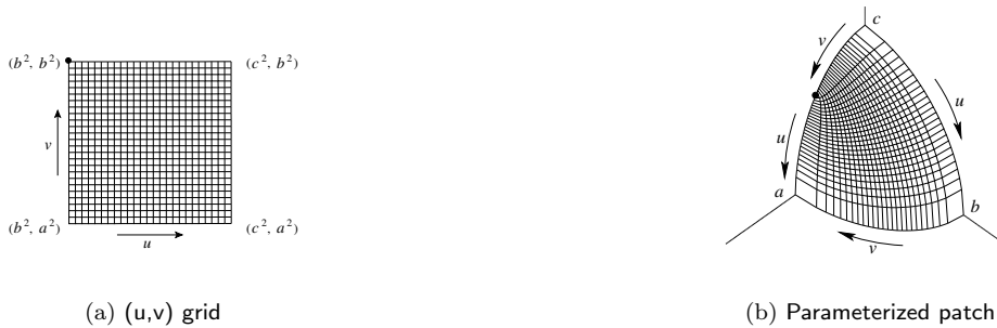
Fig. 11. Elliptic coordinates for the portion of ellipsoid in the positive octant. The parameterization is not orientation preserving, and maps the point (b^2, b^2) to the corner of the cusp in (b).
