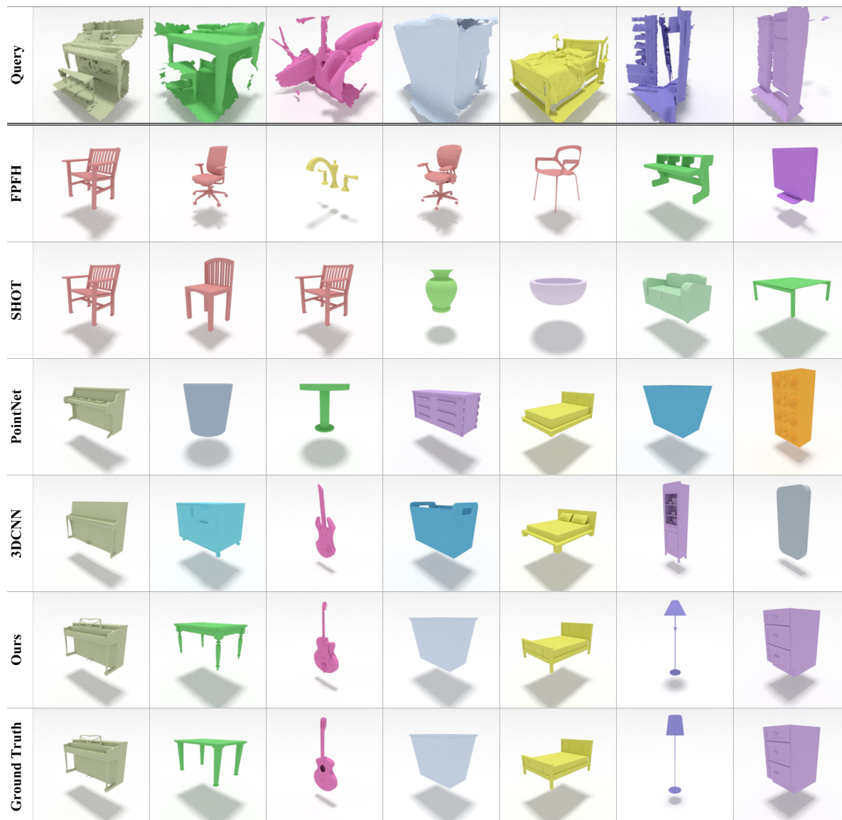
Figure 5: CAD model retrieval results (top-1) for various scan queries (from left to right: piano, table, guitar, trash bin, bed, lamp, dresser). Our approach to a joint embedding of scan and CAD can retrieve similar models at a finer-grained level than state-of-the-art handcrafted (FPFH [27], SHOT [29]) and learned (PointNet [25], 3DCNN [26]) 3D object descriptors.
