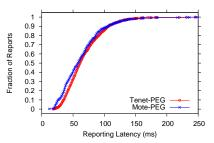
Figure 9—PEG detection latency
