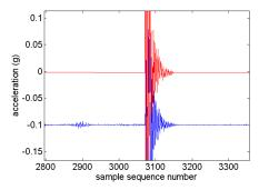
Figure 11—Vibration sensing with onset detector
