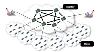
**Figure 1**—A tiered embedded network. Note that tiering does not imply physical clustering; some motes can communicate with more than one master, possibly over multiple mote hops.
