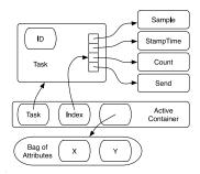
Figure 2—Mote data structures for a typical task
