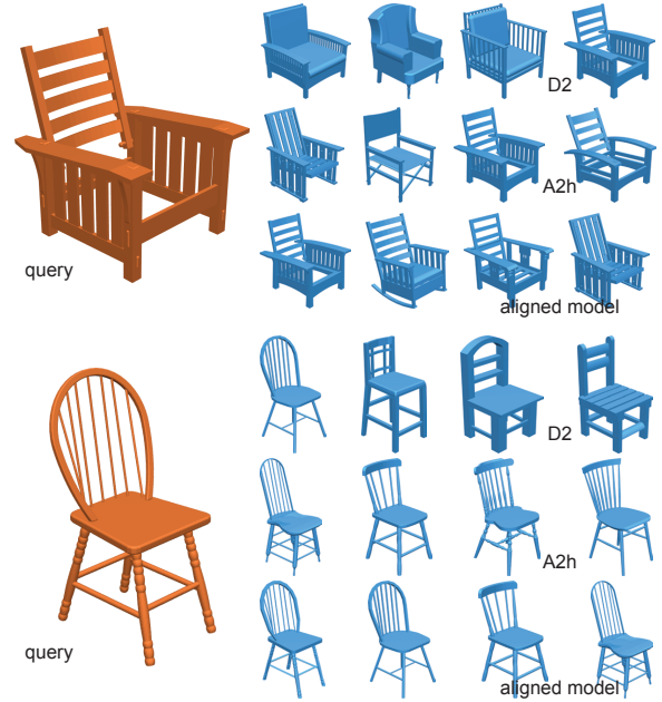
Figure 4: Representative shape retrieval results using the D2 descriptor ([OFCD02], first row), the A2h descriptor introduced in this chapter (Section 4.2, second row), and the aligned models after scan registration (Section 4.3, third row). For each method, we only show the top 4 matches. The D2 and A2h descriptor (first two rows) are compared by histogram distributions, which is a quick and efficient. Empirically, we observed the A2h descriptor to better capture local geometric features compared to the D2 descriptor, with local registration further improving the retrieval quality. The comparison based on 3D alignment (third row) is more accurate, but require more computation time, and cannot be performed in real-time given the size of our database of models.
