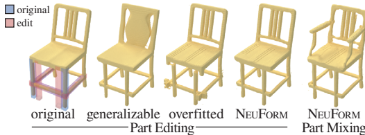
Figure 1: Adaptive overfitting. NEUFORM enables detail preserving shape edits that generalize to new part configurations by combining advantages of a generalizable representation (e.g., generation of plausible joint geometry) and an overfitted representation (e.g., detail preservation on the backrest), and also allows mixing parts from different shapes.
