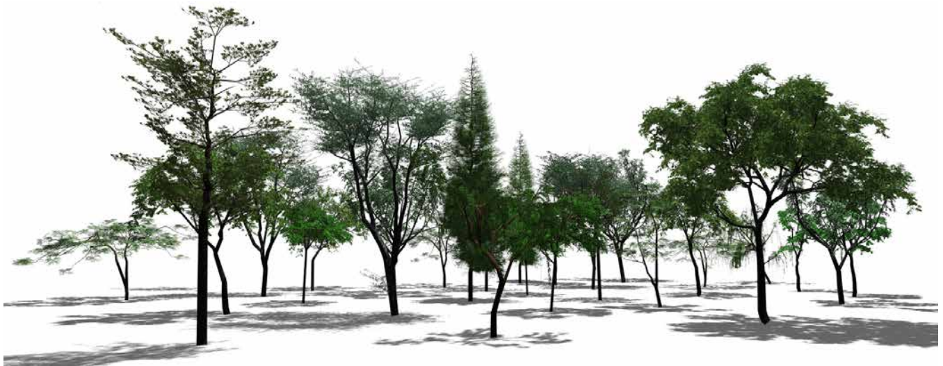
Figure 13: A large scene shown in our interactive system. Thirty trees with the intermediate lobe-based representation (250kB) are synthesized on-the-fly with a total geometry of over 40M triangles, achieving 25 fps on a standard PC using NVidia GeForce GTX 480 graphics board.
