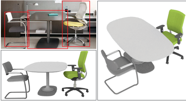
Figure 12: Interactive image-based scene modeling. Starting from an image with user-marked object bounding boxes (upper left), our system retrieves similar 3D models. Together with 3D poses estimated by [Su et al. 2015a], a 3D scene (lower left) can be modeled with a layout reasoning module from [Choi et al. 2013]. The model retrieval and pose estimation are conducted in real-time, and the user is given instant feedback once a bounding box is drawn. Equipped with such a system, 2D scene images can be easily lifted into 3D and rendered from novel views (right).
