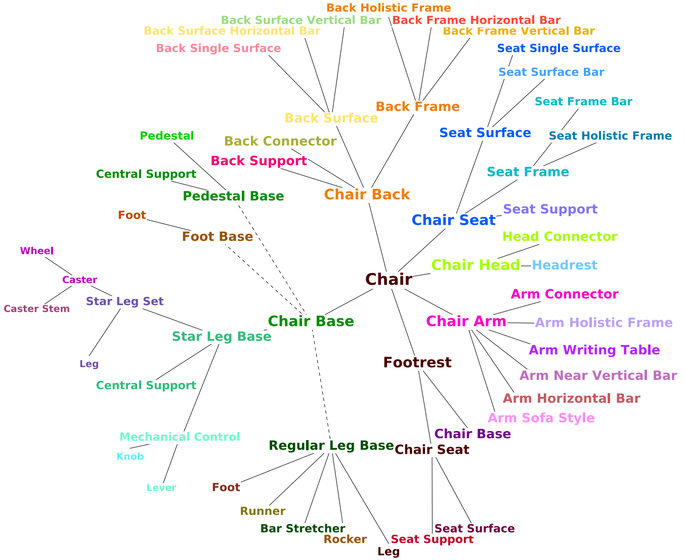
Fig. 19. PartNet semantic hierarchy for chairs. Dash lines show the OR-nodes and solid lines show the AND-nodes in PartNet. We assign the semantic labels in the figures with the colors that we use for box-shape and point cloud visualization in the main paper.
