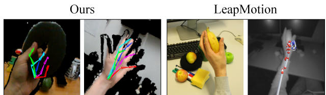
Figure 10: Fast motion that leads to misalignment in the colored depth image or failures in the hand localization step can lead to incorrect predictions (left two columns). LeapMotion Orion fails under large occlusions (right).
