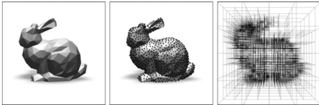
Fig. 4. We capture interactions by defining sensor regions in the domain around the observed shape (left). We compute samples on its surface (middle) and use them to produce a spatial subdivision of a graded set of cubes that get finer close to its surface. Location and size of each sensor correspond to the leaf nodes of an Octree that generates the sensor regions (right).
