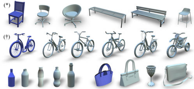
Fig. 16. Visual comparison of models retrieved by our descriptor. The query object is shown in blue, the closest models according to our descriptor to the right; the retrieved objects share similar properties in descending order. The motion drivers used for this experiment were: sitting animation (chairs), fluid simulation (bicycles), grasping simulation (bottles, bags).
