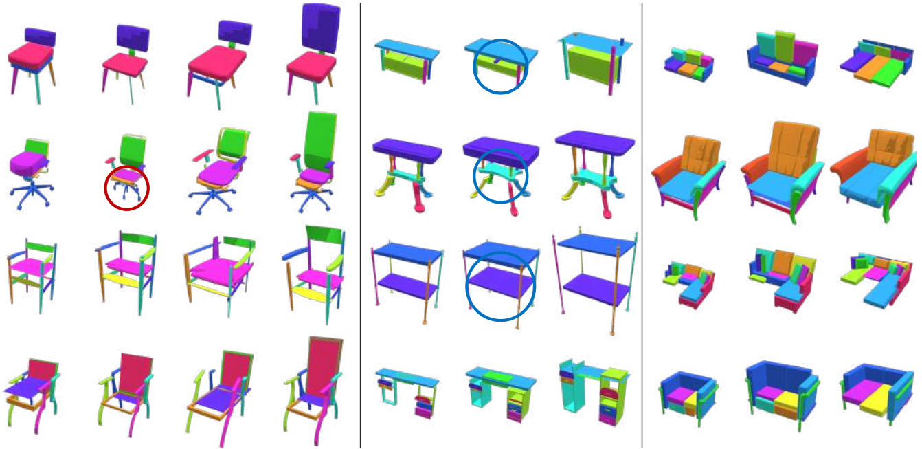
Fig. 5. Elements in the learned deformation dictionary. The columns are deformations along some elements in the dictionary (columns of A_x ). Each element shows a natural mode of shape variations changing local parts, and the variations of each element are also consistent across the shapes despite the difference in styles of the shapes. The second column of chairs shows scaling of swivel leg (red circle), and the element does not affect the shapes not including the swivel leg. Also, the second column of tables lifts up the shelf in the middle (blue circle) and makes no change if the part does not exist. Refer to the supplemental video for animated visualizations.
