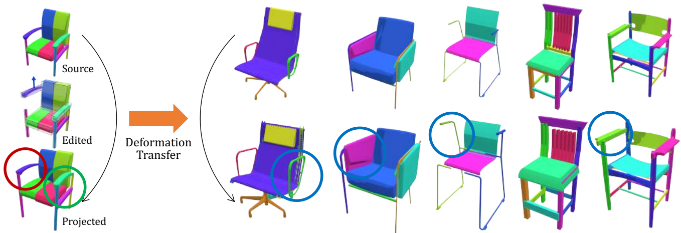
Fig. 1. We propose DEFORMSYNCNET to jointly learn an idealized canonical latent space, encoding all possible deformations from one shape to any other, as well as an individualized linear deformation space, realized in a particular way for each specific shape. These individual deformation spaces are synchronized via the connection to the canonical space, resulting in consistent deformations across an entire shape category. Here, a user’s manipulations on a shape is projected to a learned plausible shape space (left) while maintaining the shape structure such as part connectivity (red circle) and symmetry (green circle) and also instantly transferred to multiple other shapes from the same category (right), without leveraging any correspondence information during network training. Note how the edit only affects the other chairs with arms (blue circle).
