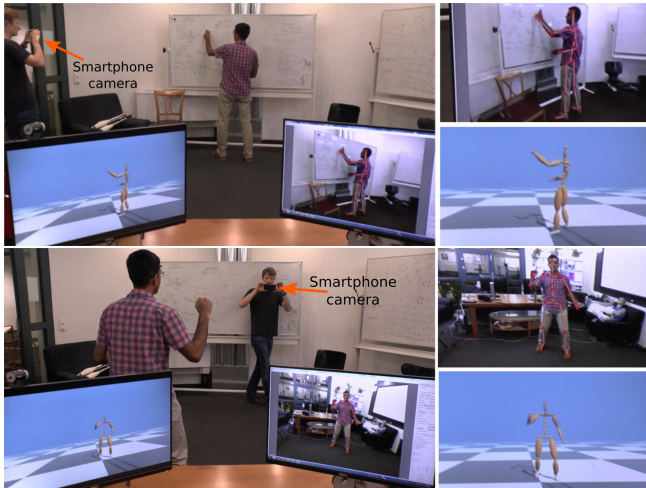
Fig. 15. Handheld recording with a readily available smartphone camera (left) and our estimated pose (right), streamed to and processed by a GPU enabled PC.
