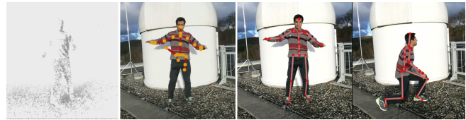
Fig. 7. Our approach succeeds in strong illumination and sunlight (center right and right), while the IR-based depth estimates of the Microsoft Kinect are erroneous (left) and depth-based tracking fails (center left).
