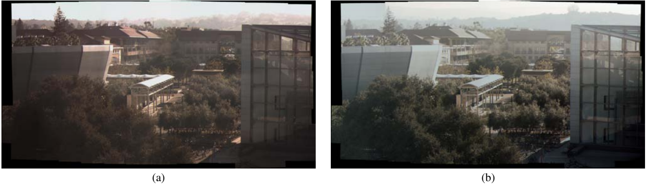
Figure 6: High Dynamic Range Panoramic Video. By metering cameras individually, we can increase the total dynamic range of the panoramic video. (a) In this image, all cameras are set to the same exposure. Notice the saturated areas in sunlight and dark regions in shade. (b) For this mosaic, each camera's exposure was set such that the average pixel value is in the middle of the sensor range, and the resulting high dynamic range image was tone mapped for display (and printing). More details are revealed, including the radar dish and hills on the horizon and dark areas in the foreground trees. The roof of the covered walkway, however, was outside the range of the cameras that viewed it. The gray color is due to tone mapping—we do not actually know how bright the roof should be. The sky in the top left of the panorama was also overexposed.
