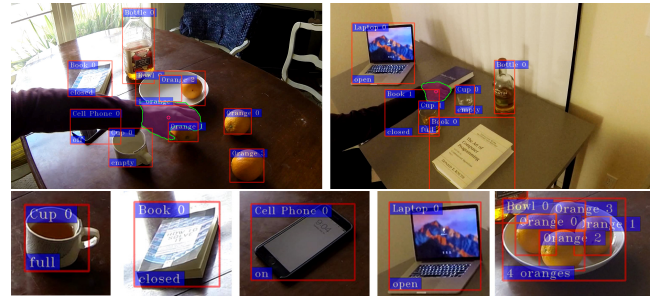
Figure 5: Top row: two results of our tracking pipeline; our method is able to detect the type, state, and instance of objects and to segment articulated hand masks (blue overlay, green border). Bottom row: we detect object states using SVM classifiers and represent them as discrete stages.
