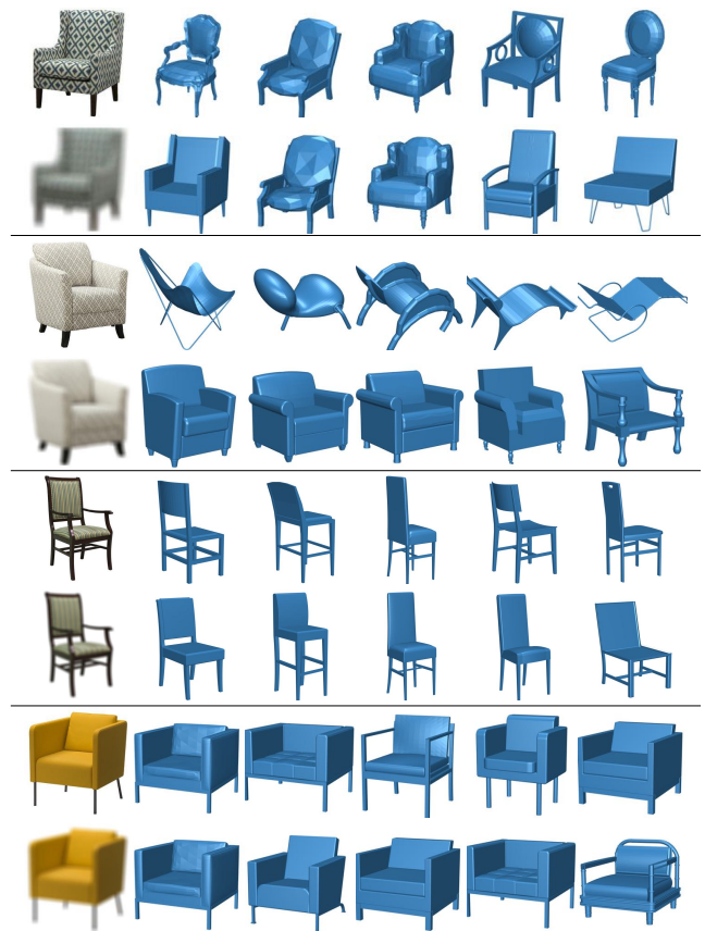
Figure 4: Shape retrieval and alignment. Here we show 5 closest results of original and blurred image (to reduce texture effects). We use the closest shape (second column) for further estimation. For each image, we use the estimated view corresponding to the model in the second column.
