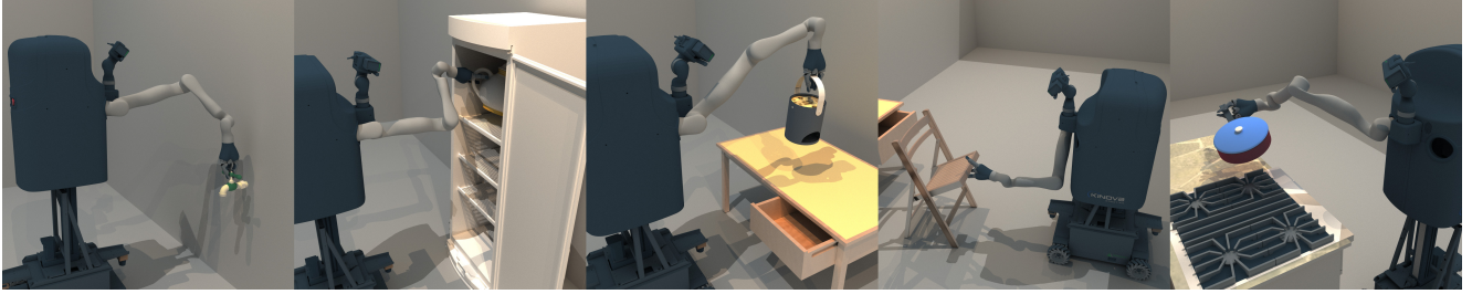
Figure 3: SAPIEN Enables Many Robotic Interaction Tasks. From left to right, we show five examples: faucet manipulation, object fetching, object lifting, chair folding, and object placing.
