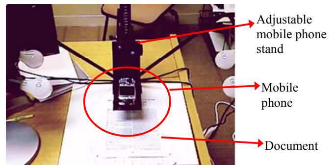
Figure 9. Device for capturing and ground truth.
