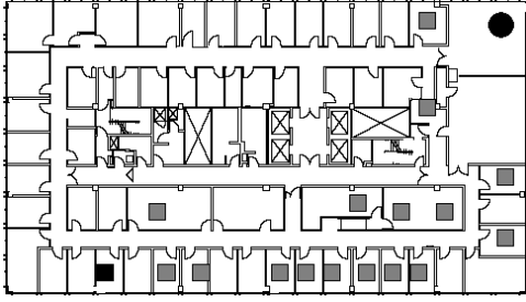
Fig. 6: Testbed deployment map. Gray boxes are relay nodes. The black circle (top-right) is a source node. The black box (bottom-left) is a sink node.
