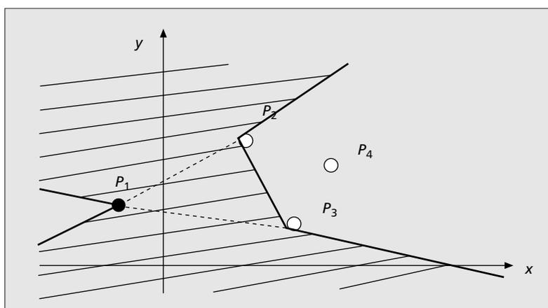
■ **Figure 6.** An estimation of the location of the shadow edge, subject to the resolution of the sensor field.
