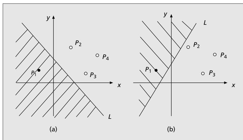
■ **Figure 4.** Two different configurations that yield the same sensor reading.
