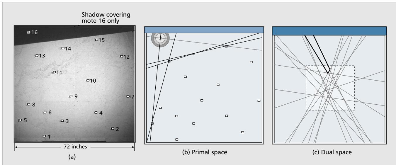
**Figure 8.** a) A testbed contains 16 motes mounted on a board; a half-plane shadow is cast onto the board; b) the detection and estimation of the shadow edge; c) the dual-space representation of the corresponding cell. Motes 16, 15, 14, 13, and 5 are the current frontiers for detection.
