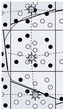
A wireless network of sensors can cover a large geographical region, and hence can be used to detect and track non-local phenomena which cannot be captured by any individual sensor.
