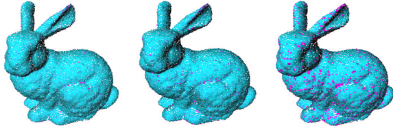
Figure 7: Normal estimation errors for the bunny PCD with noise added. The subfigures show the points of the PCD using the pink color whenever the errors are above 10^\circ , 8^\circ , and 5^\circ respectively.
