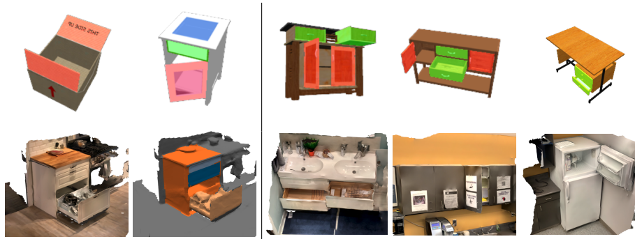
Fig. 2: Example articulated objects from the OPDSynth dataset and the OPDReal dataset. The first row is from OPDSynth. Left: different openable part categories (lid, in orange, drawer in green, door in red). Right: Cabinet objects with different kinematic structures and varying numbers of openable parts. The second row is from our OPDReal dataset. Left: reconstructed cabinet and its semantic part segmentation. Right: example reconstructed objects from different categories.
